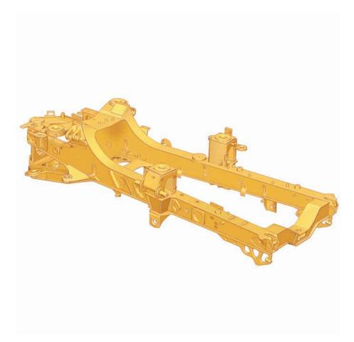
Hitch Construction. Two-piece hitch construction features a strong, durable cast steel head bolted to a hard wearing forged steel tube. The hitch tube has large, hardened bearing areas and a hardened thrust face for reduced maintenance and longer life.
